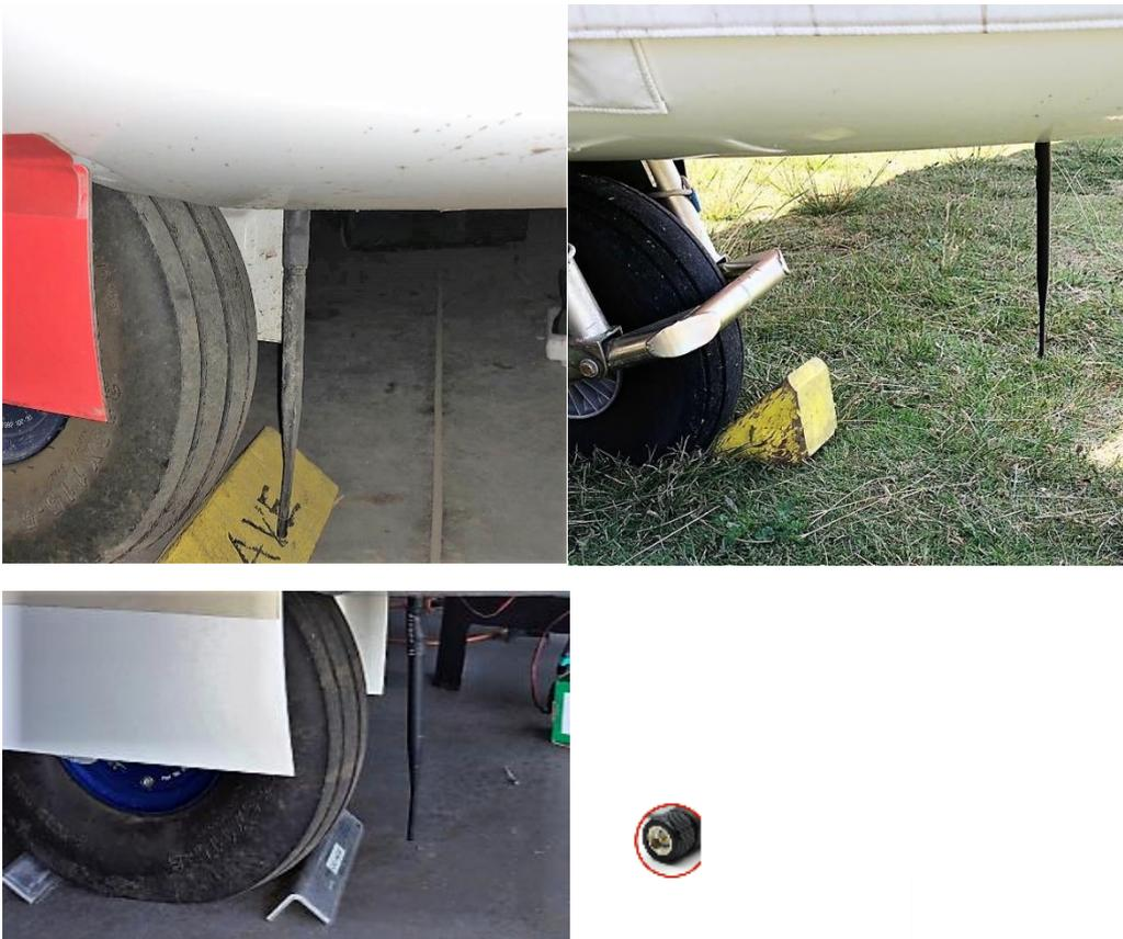
The antenna has a SMA male connector see picture above, so the termination of the cable has to be female connector going to the antenna and a termination SMA male connector going to the OGN/IGC tracker.
