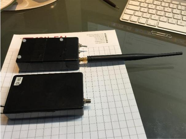
The external antenna will be connected to the OGN/IGC tracker provided by the organization. For the Flarm unit we recommend to have a similar antenna inside the cockpit. In Europe the Flarm/OGN frequencies are on the **ISM band (868.2 MHz) unique frequency, so we require an antenna for that frequency with at least 3dbi or better**, and we recommend the following antennas:
