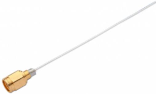
The antenna has to be placed below the cockpit pointing down and requires a 7 mm diameter hole on the fuselage (the drain hole could be used for this purpose), the antenna is connected to a coaxial cable (**50 ohm**, we recommend Aircell7 or Ecoflex10 given the frequencies that we use) to the OGN/IGC tracker external antenna SMA male connector.
